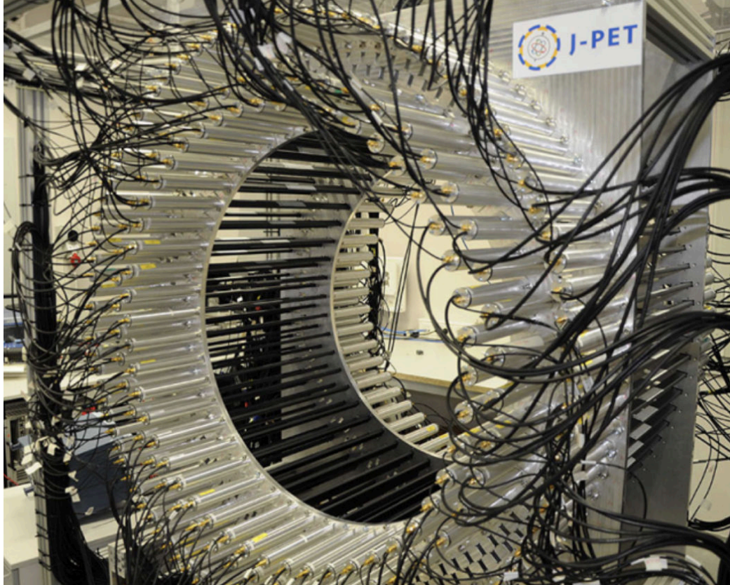
Rysunek 3.2: The first large scale prototype of the J-PET constructed in the tree layers arrangement of the plastic scintillator (back) coupled with PMT at each end (silver).
