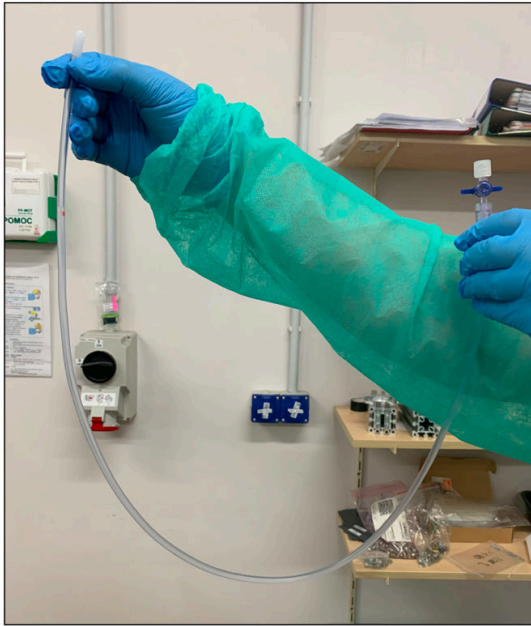
Rysunek 7.4: (Right ): Display the 70 cm tube that uniformly filled with a water solution containing ^{18}\text{F} isotope with a well defined activity. (Left): Schematic decay of the ^{18}\text{F} . Figure adapted from [112].
