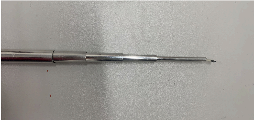
Rysunek 4.1: Sensitivity Phantom with five sleeve tubes and one polyethylene tube (sixth layer) with length of 70 cm.
