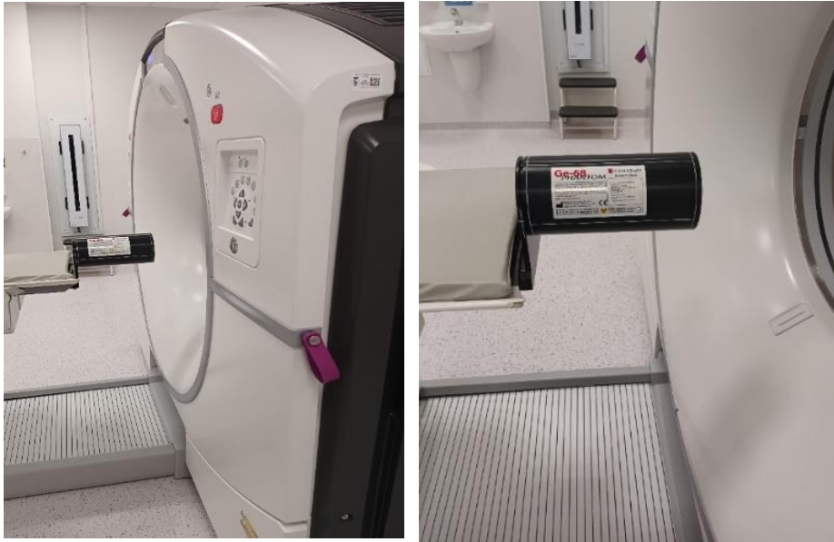
Figure 2. 6 Dedicated source ^{68}\text{Ge}/^{68}\text{Ga} for quality control of PET/CT system.
