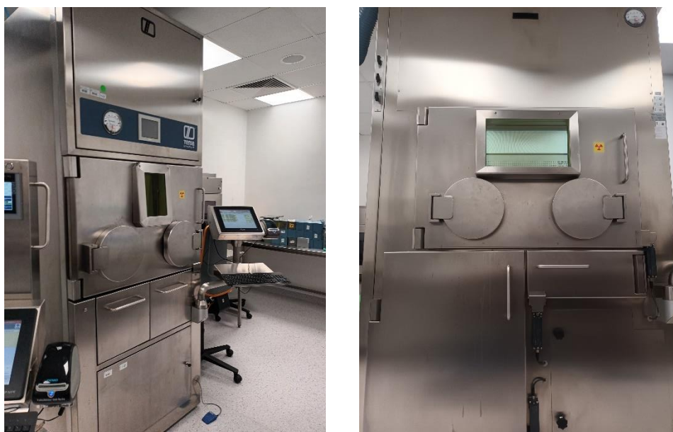
Figure 2. 2 Hot cell for radiolabeling radiopharmaceuticals.
